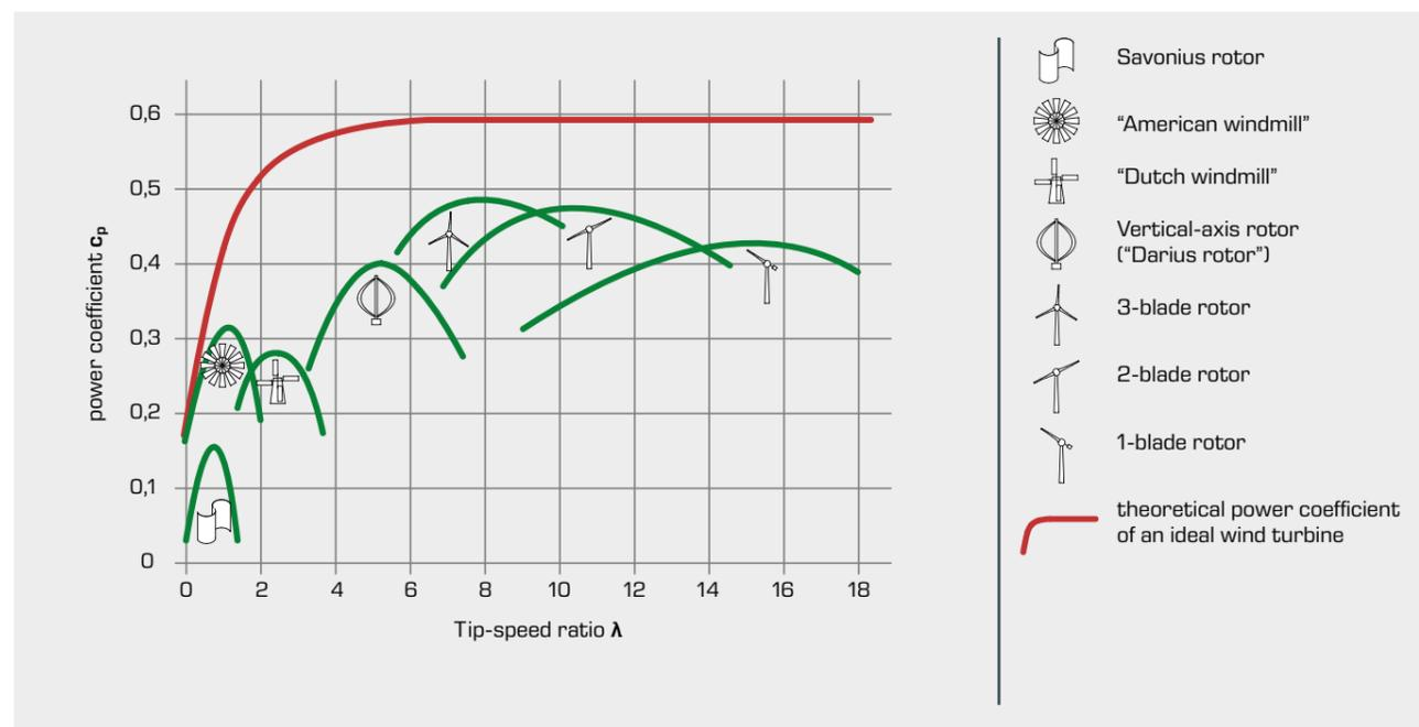
The higher the tip-speed ratio, the better the aerodynamic rotor blade profile must be. Otherwise the drag forces would have a counter-effect on any possible high power coefficients.
