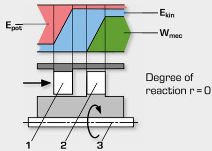
**Action turbine:** In the distributor, the potential pressure energy is completely converted into kinetic energy. The rotor then converts the kinetic energy into mechanical work.
