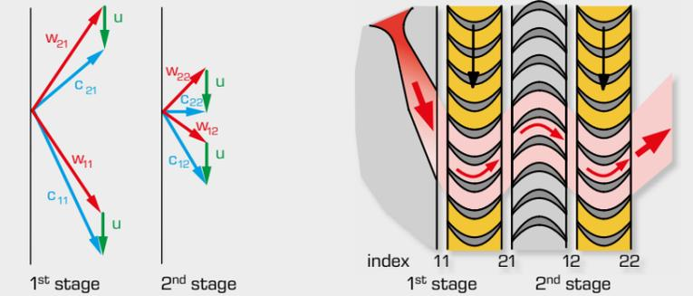
**Reaction turbine with pressure stages:**
