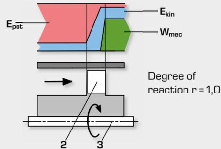
**Pure reaction turbine:** The conversion of the potential pressure energy into kinetic energy takes place in only one nozzle in the rotor. The recoil of the nozzle then provides the impulse for the mechanical work. Pure reaction turbines are not used in industrial applications. The figure represents an abstract form.
