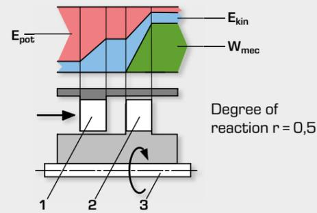
**Reaction turbine:** The conversion of the potential pressure energy is divided among the distributor and rotor. The kinetic energy is then converted into mechanical work at the rotor.
