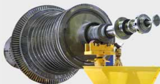
Disassembled steam turbine rotor
