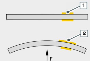
F force, 1 strain gauge in component not under load, 2 strain gauge in component under load
