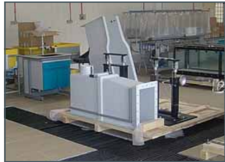
Inlet element, outlet element and flume supports
