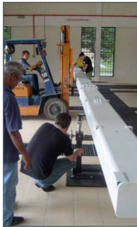
The carrier (bottom left) is assembled from separate elements (left) and placed on the flume supports using a forklift (right). The flume supports are bolted into the floor (centre).
