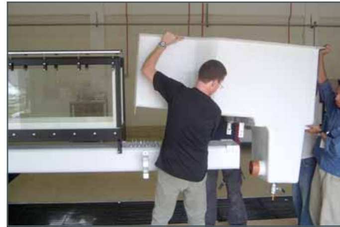
The inlet element is raised onto the carrier, aligned and connected to the experimental section.
