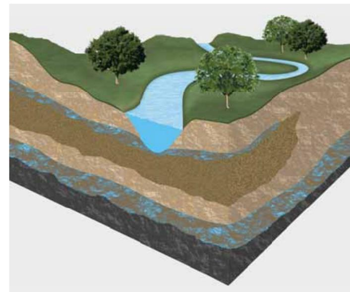
Seepage flows and groundwater flows are water movements in a permeable subsoil (sand, gravel, etc.) This includes the seepage and retention of precipitation. In hydraulic engineering it is the seepage through earth dams or the seepage under barrages in particular that are of importance.
