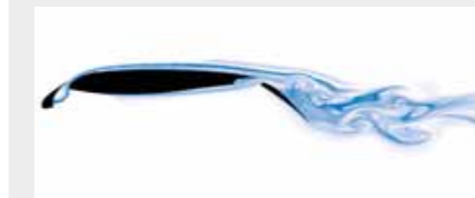
Boundary layer and flow separation on an aerofoil and landing flap
