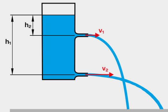
$h$  head, distance between discharge and water level,  $v$  velocity
