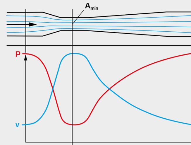
■ velocity, ■ static pressure curve
