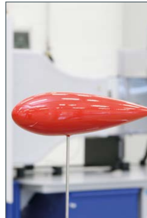
Measuring lift and drag forces on the streamlined body with the two-component force sensor
