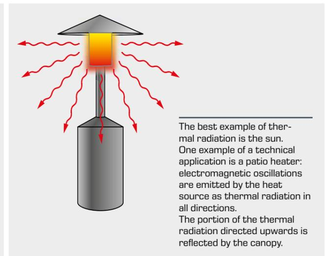
The best example of thermal radiation is the sun. One example of a technical application is a patio heater: electromagnetic oscillations are emitted by the heat source as thermal radiation in all directions. The portion of the thermal radiation directed upwards is reflected by the canopy.
