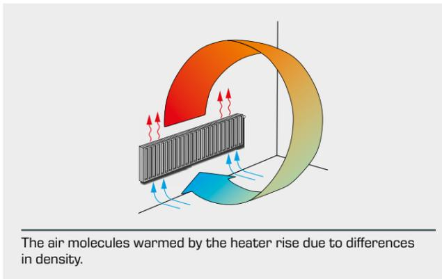
The air molecules warmed by the heater rise due to differences in density.
