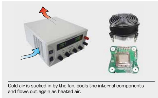
Cold air is sucked in by the fan, cools the internal components and flows out again as heated air.
