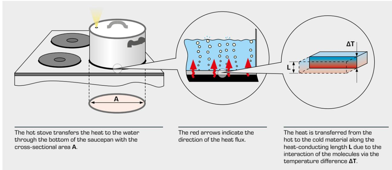
The hot stove transfers the heat to the water through the bottom of the saucepan with the cross-sectional area  $A$ .
