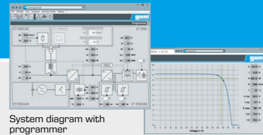
Simulated characteristic curve with ET 255.01 photovoltaic simulator
