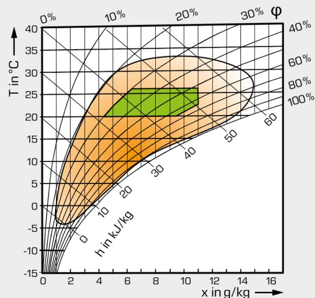
In the h-x diagram temperature  $T$ , enthalpy  $h$  and relative humidity  $\phi$  are plotted above the absolute humidity  $x$ .
