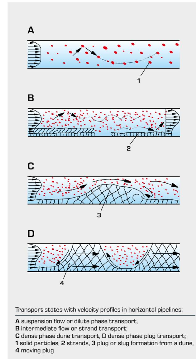
Depending on the velocity and solid content of the airflow, different transport states may occur in **horizontal** pipelines:
