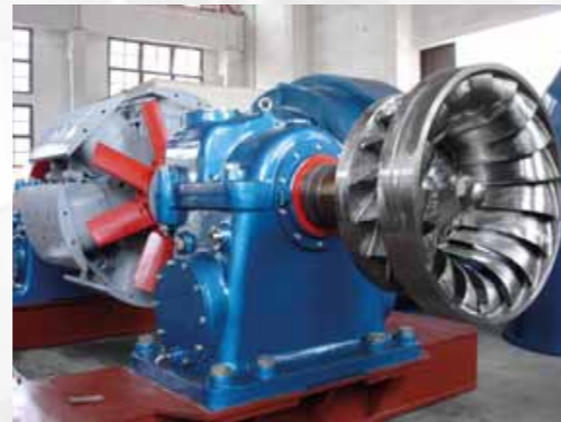
Francis turbine, deinstalled
