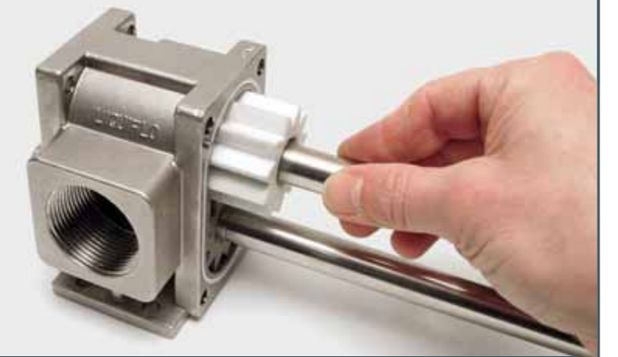
MT 186 Assembly & maintenance exercise: gear pump
