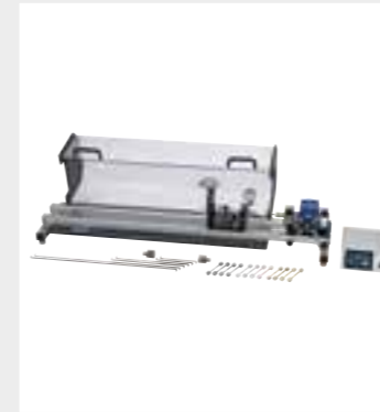
The compact WP 500 experimental unit generates reference moments of 30Nm
