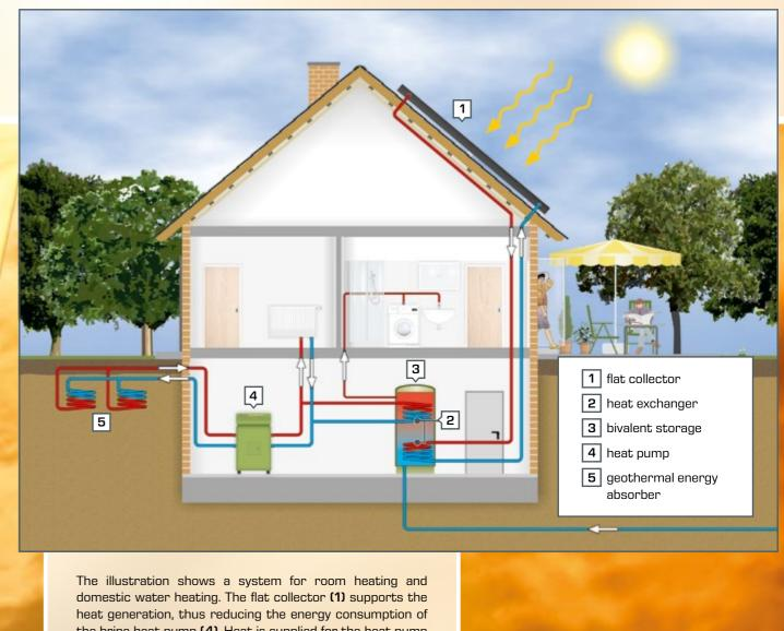
the brine heat pump (4). Heat is supplied for the heat pump by the geothermal heat absorber (5). The bivalent storage (3) enables integration of different heat sources and creates a balance between heat supply and demand.
