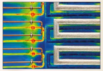
The insulation of heat transfer conduits also provides a significant contribution to energy efficiency.
