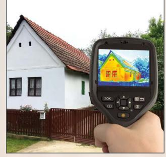
A lack of insulation in old buildings can lead to heat leakages. These problem areas can be detected by means of sensitive infrared cameras based on the emitted heat radiation. It is not just the heat conduction of materials, but also how they are fabricated that determine the effectiveness of insulation in walls and heat transfer conduits.
