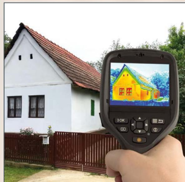
A lack of insulation in old buildings can lead to heat leakages. These problem areas can be detected by means of sensitive infrared cameras based on the emitted heat radiation. It is not just the heat conduction of materials, but also how they are fabricated that determine the effectiveness of insulation in walls and heat transfer conduits.
