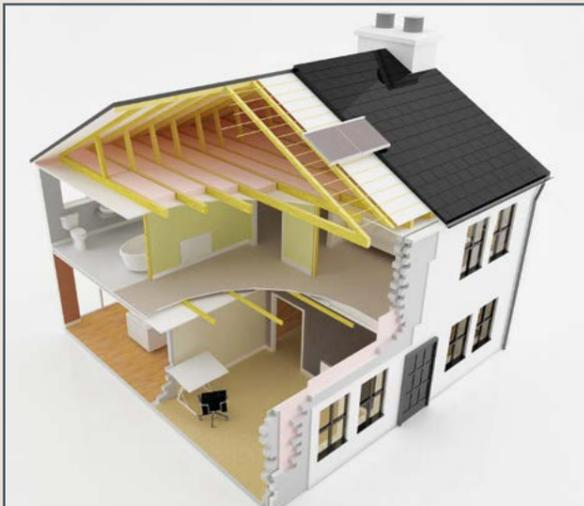
Improving the thermal insulation of walls and roofs is only one possible measure towards energy savings in buildings. An economic assessment requires an analysis of the savings to be expected through reduced heat losses in each individual case.
