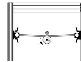
Investigation of **forced vibration** by an imbalance exciter; controllable frequency and imbalance exciter amplitude
