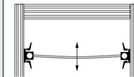
**Elastic bar** as oscillating continuum, either fixed or movable support, ball-bearing-mounted for minimal system damping
