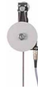
Tunable vibration absorber for investigating **vibration-absorbing effects**
