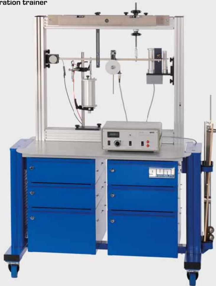
To study **pendulums**, the trainer includes different pendulum versions and a pendulum bearing:
