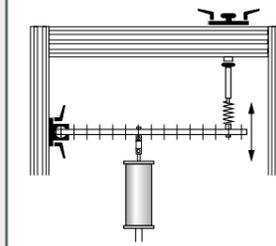
**Rigid bar** as discrete rotational oscillator, fixed support, suspension on a helical spring. A breadboard allows the attachment of springs, exciters and absorbers in a wide variety of reproducible configurations.
