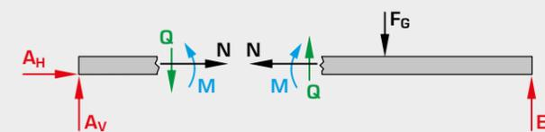
$F_G$  weight,  $q$  snow load,  $A$  and  $B$  support forces, **index V** vertical forces, **index H** horizontal forces,  $N$  normal force,  $Q$  shear force,  $M$  bending moment
