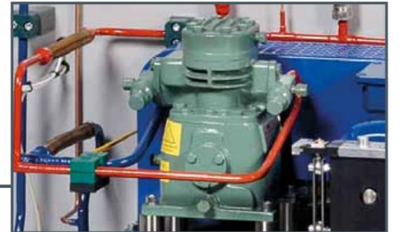
The **compressor** is the drive unit of a compression refrigeration system. It extracts the gaseous refrigerant from the evaporator, increases the pressure of the refrigerant vapour and conveys the gaseous refrigerant into the condenser. The compressor must raise the pressure of the refrigerant vapour to a sufficiently high pressure level so that the refrigerant can condense in the condenser by releasing heat.
