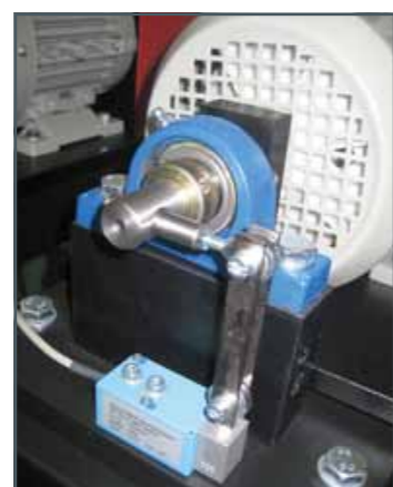
Each pump testing station has a measuring device for detecting the drive torque
