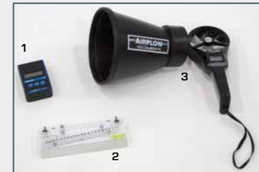
1 digital manometer, 2 inclined tube manometer, 3 anemometer
