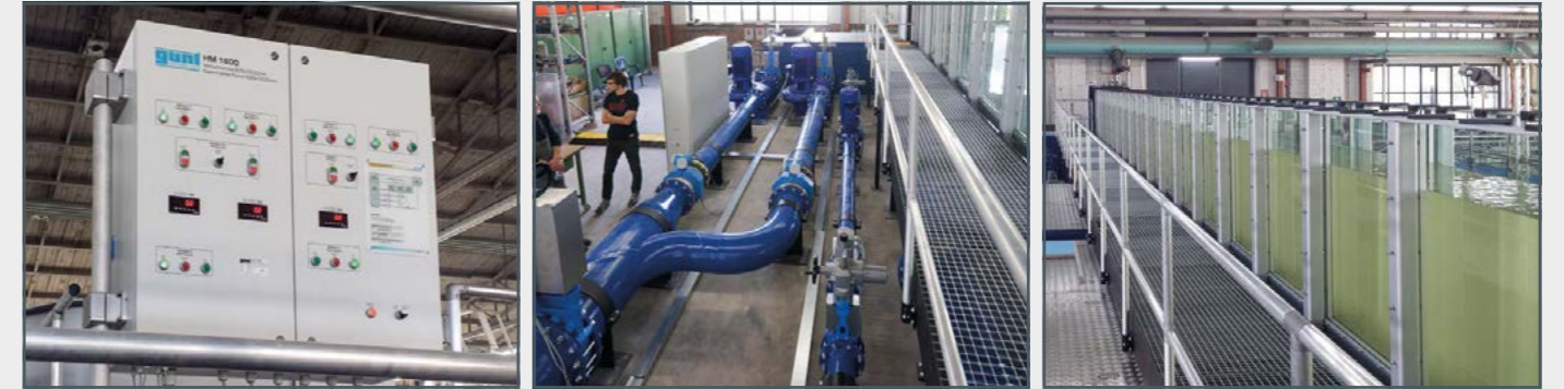
HM 1600 Flow channel 600x1200 mm, 20 m length
