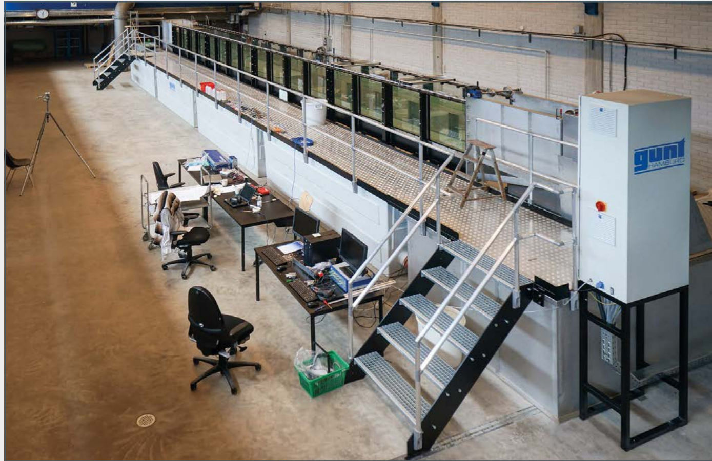
HM 161.FI Flow channel 600x800 mm, 16 m length
