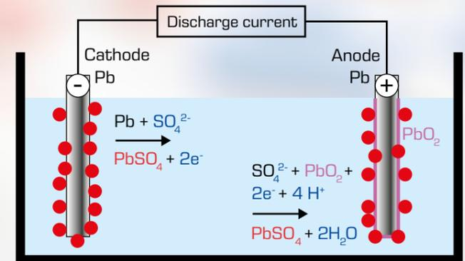
The illustration shows the sub-reactions during discharge of a lead accumulator
