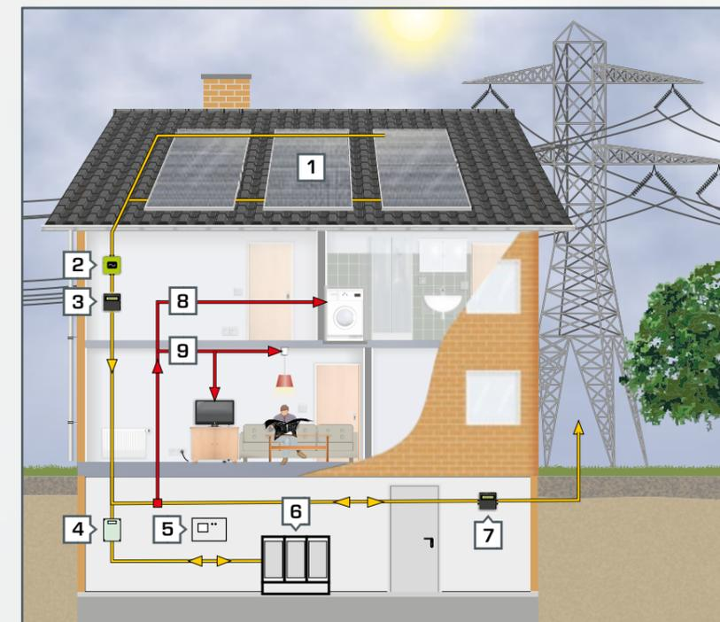
Increasingly larger battery storage systems are also planned as part of grid-connected photovoltaic installations. Consequently it is possible to increase in-house consumption and to reduce the extraction of electricity from the grid.
