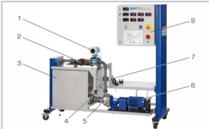
1 electromagnetic flow meter, 2 flow control valve, 3 storage tank, 4 pressure sensor at pump inlet, 5 centrifugal pump, 6 drive motor including measurement of torque, 7 pressure sensor at pump outlet, 8 switch cabinet with displays and controls
