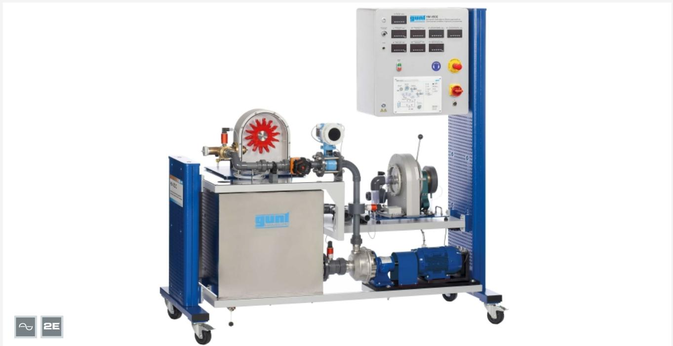
The illustration shows HM 450C together with the turbines HM 450.01 (left) and HM 450.02 (right).
