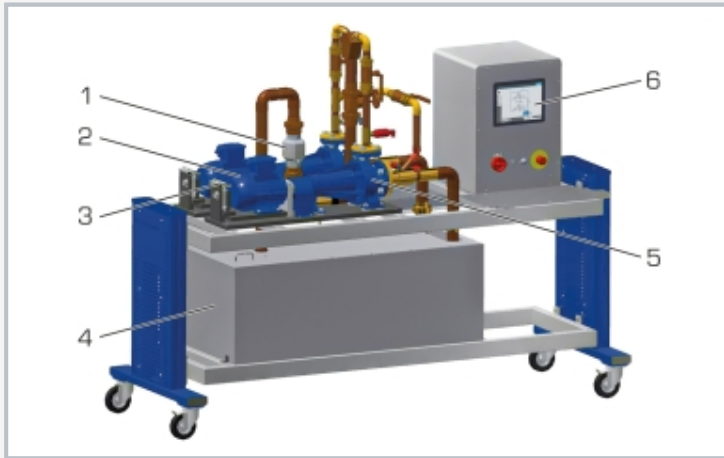
1 electromagnetic flow meter, 2 drive motor, 3 force sensor, 4 storage tank, 5 pump, 6 touch screen
