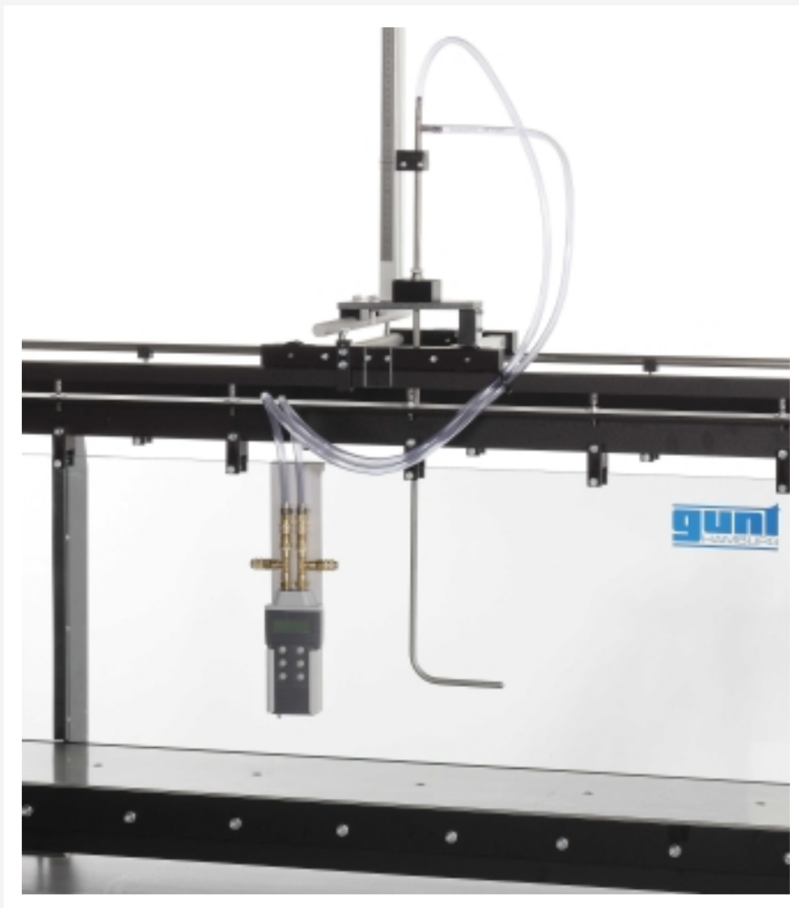
The illustration shows a similar pitotstatic tube mounted onto an instrument carrier
