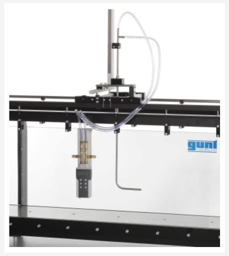
The illustration shows a similar pitotstatic tube mounted onto an instrument carrier
