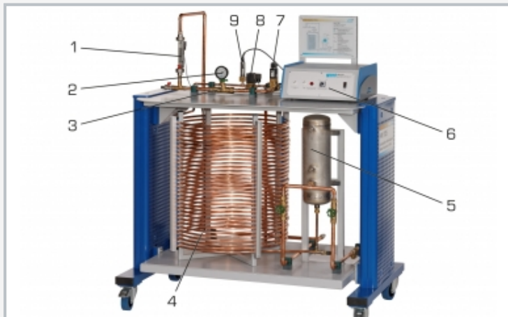
1 flow meter, 2 manometer, 3 valve for flow rate adjustment, 4 pipe section, 5 pressure vessel, 6 control unit, 7 adjustable solenoid valve, 8 constant solenoid valve, 9 pressure sensor
