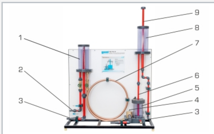
1 inlet tank with fixed overflow, 2 water connection, 3 water discharge, 4 waste valve with lift, 5 air vessel with air volume and non-return butterfly valve, 6 riser, 7 pipe, 8 elevated tank, 9 adjustable overflow
