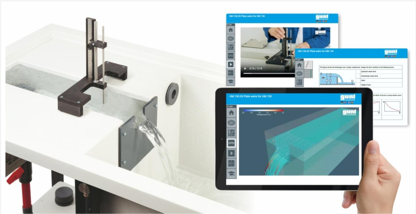
The illustration shows the HM 150 base module with built-in Rehbock weir and the GUNT Science Media Center, tablet not included.
