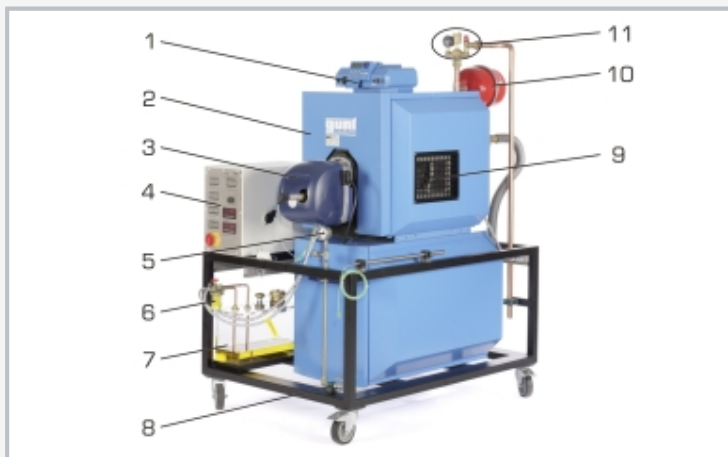
1 heating control unit, 2 heating boiler, 3 HL 352.01 Oil burner [not included], 4 switch cabinet with digital displays and control panel, 5 gas pressure manometer, 6 two-strand oil filter, 7 fuel oil tank with fittings, 8 gas connection, 9 viewing window in the heating control, 10 expansion tank, 11 boiler safety group
