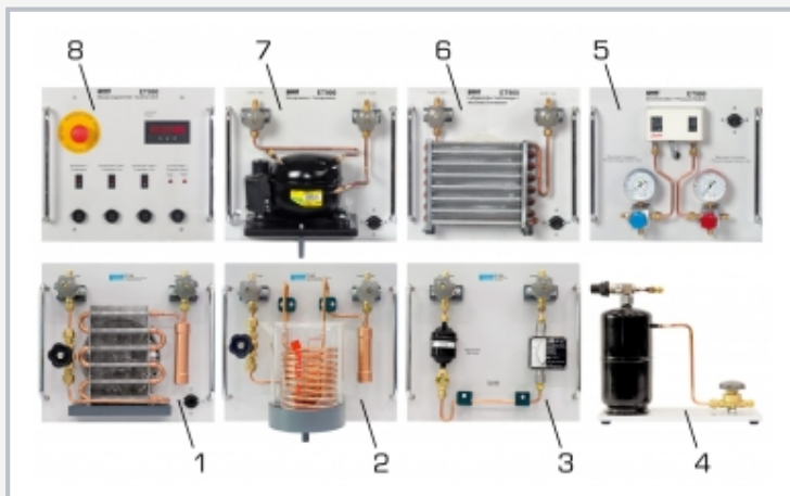
1 air cooling evaporator, 2 water cooling evaporator, 3 sight glass with filter/drier and flow meter, 4 receiver, 5 pressure switch, 6 air-cooled condenser, 7 compressor, 8 display and control panel
