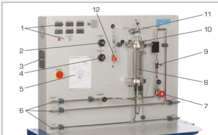
1 displays and controls, 2 valve for sealing steam, 3 steam connection, 4 valve for steam inlet, 5 process schematic, 6 water connections, 7 pressure sensor for condensate measurement, 8 condenser with coil, 9 cooling water flow rate sensor, 10 turbine, 11 eddy current brake, 12 pressure sensor
