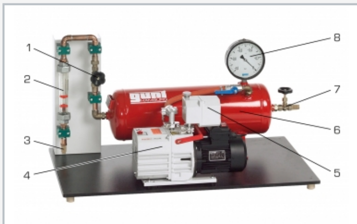
1 needle valve, 2 flow meter, 3 silencer, 4 rotary vane pump, 5 oil separator, 6 pressure vessel, 7 needle valve with silencer, 8 manometer
