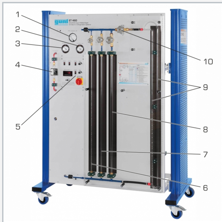
1 manometer differential pressure, 2 manometer delivery side, 3 manometer intake side, 4 flow meter, 5 display and control elements, 6 rising pipe Ø 6mm, 7 rising pipe Ø 10mm, 8 rising pipe Ø 14,4mm, 9 double rising pipe, 10 valve for rising pipe selection
