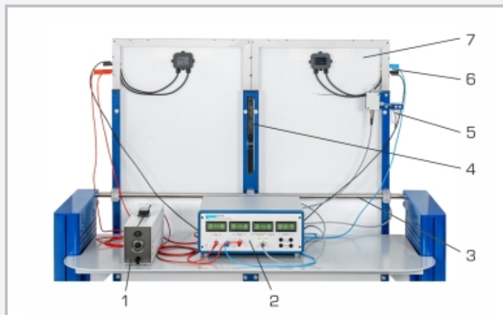
1 slide resistor, 2 measuring amplifier, 3 inclination axis for inclination adjustment, 4 inclinometer, 5 illuminance sensor, 6 temperature sensor, 7 photovoltaic modules
