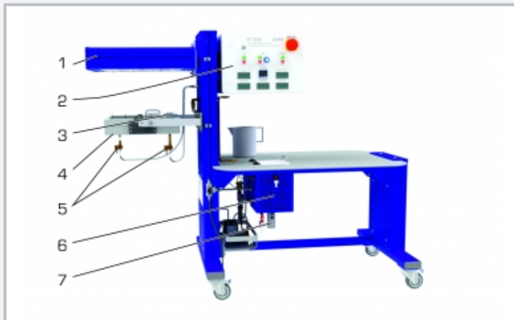
1 lighting unit, 2 control cabinet, 3 illuminance sensor, 4 flat collector with spacing and inclination adjustment, 5 temperature sensor, 6 hot water storage tank, 7 electrical auxiliary heater
