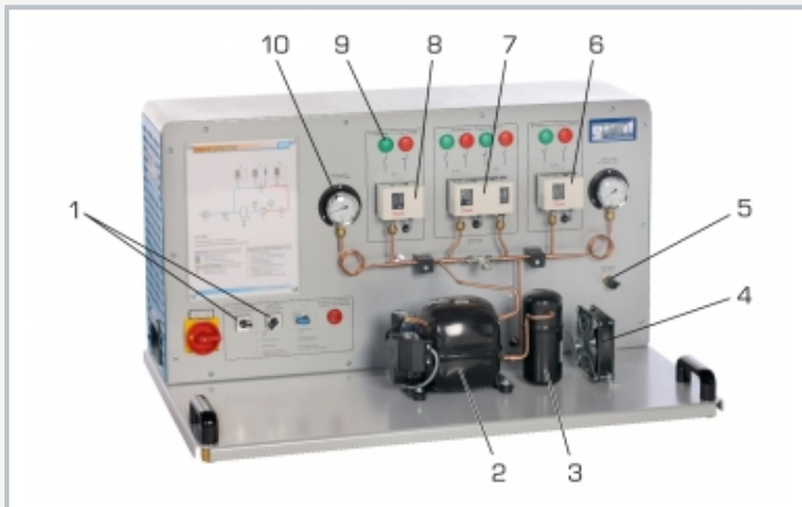
1 controls, 2 compressor, 3 receiver, 4 fan, 5 vent valve, 6 high pressure pressure switch, 7 combined pressure switch, 8 low pressure pressure switch, 9 signal lamps for switching state, 10 manometer
