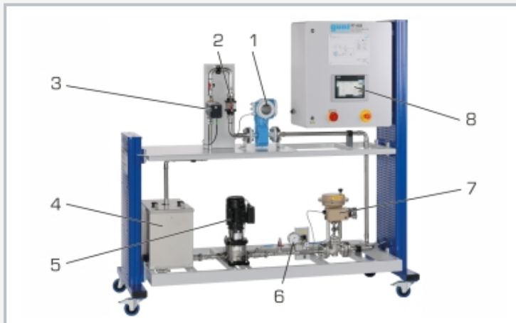
1 smart flow rate sensor, 2 flow rate indicator, 3 proportional valve with motor drive, 4 storage tank, 5 pump, 6 manometer, 7 control valve, 8 touch screen
