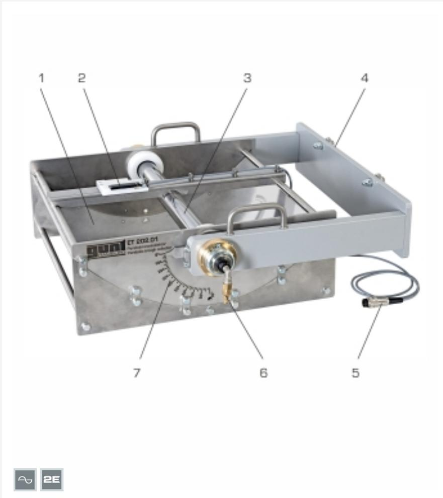
1 parabolic trough mirror, 2 illuminance sensor (scope of delivery of ET 202), 3 absorber tube, 4 suspension, 5 sensor cable and connection (scope of delivery of ET 202), 6 connection to solar circuit in ET 202, 7 scale
