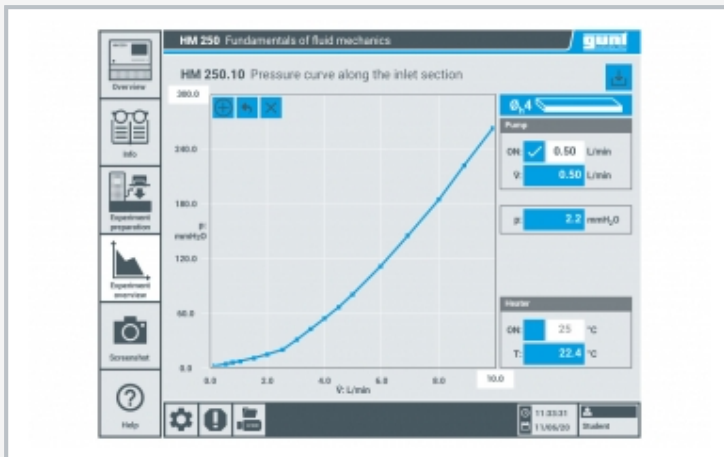
Intuitive user interface in the HM 250 touch screen: pressure measuring at pipe section (rectangular cross-section) and graphic display of the measured values, pressure curve in the formed flow area
