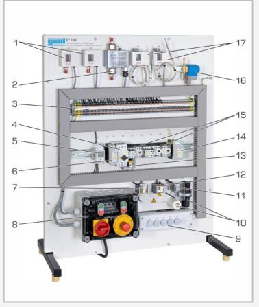
1 pressure switch, 2 differential pressure switch, 3 terminal block, 4 circuit breaker with start-up current limiter, 5 timer, 6 thermistor circuit breaker, 7 PTC start-up relay, 8 switch cabinet, 9 lamps, 10 capacitors, 11 bimetallic circuit breaker, 12 electromagnetic start-up relay, 13 adjustable protection relay, 14 time relay, 15 contactor, 16 solenoid valve, 17 thermostat
