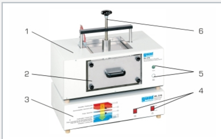
1 insulating housing, 2 cover for sample chamber, 3 control unit, 4 main switch and heater switch, 5 indicator lights, 6 contact spindle
