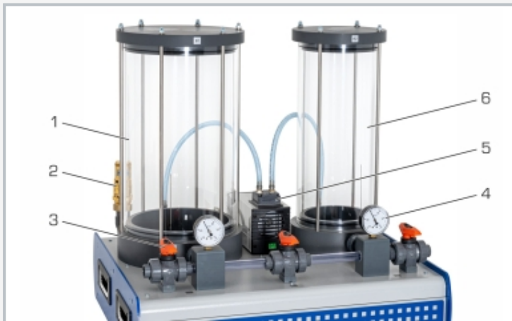
1 positive pressure tank, 2 safety valve, 3 ball valve, 4 manometer, 5 compressor, 6 negative pressure tank
