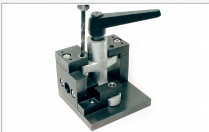
Drilling jig in use
