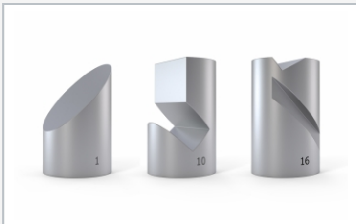
Cylindrical models with cuts parallel and oblique to the spatial axes
