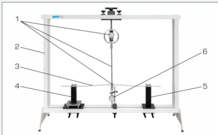
1 load application device, 2 SE 112 frame, 3 beam, 4 floating bearing, 5 fixed support, 6 dial gauge
