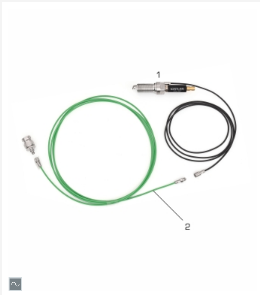
1 spark plug with pressure transducer, 2 connecting cable
